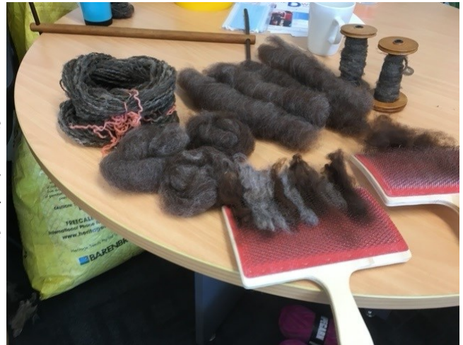
Fleece on a hand carder (front), which is carded into rolags (centre back) for spinning on a wheel onto a bobbin. Spun yarn on two bobbins (on the right), which are reverse spun together into plied wool (back left) ready for knitting.
